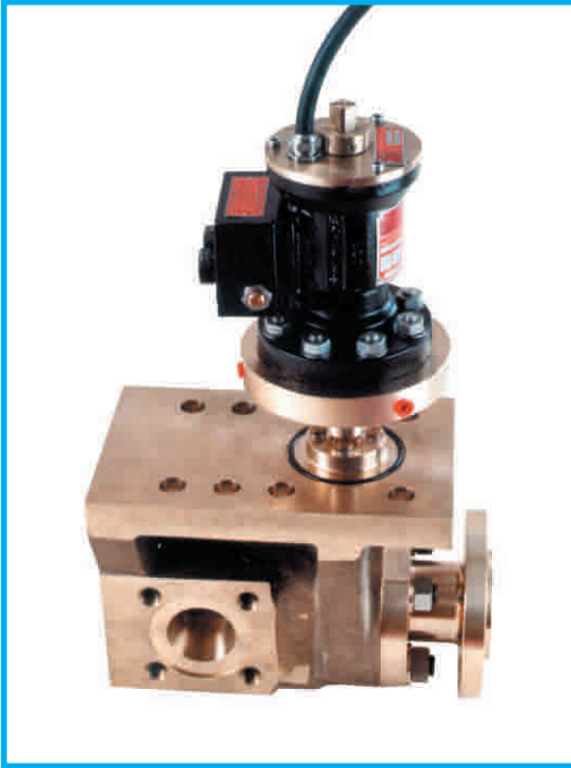
50mm Class 1 nickel aluminium bronze submarine ballast tank valve fitted with hydraulic operated actuator.
