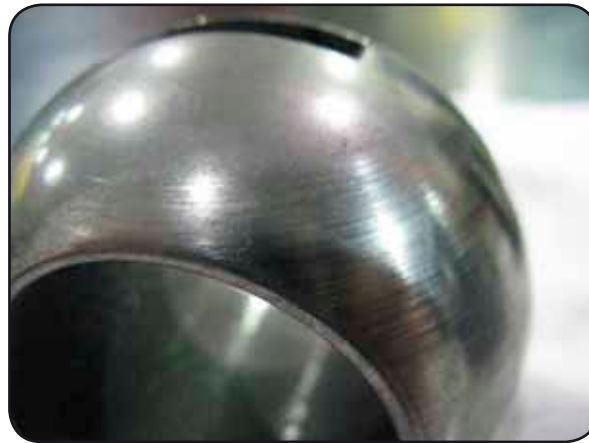
Fig 4. Cycle tested Worcester Controls Ball valve ball (© Flowserve Corporation)
