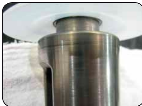
Fig 5. Cycle tested Durco Plug valve plug (© Flowserve Corporation)
